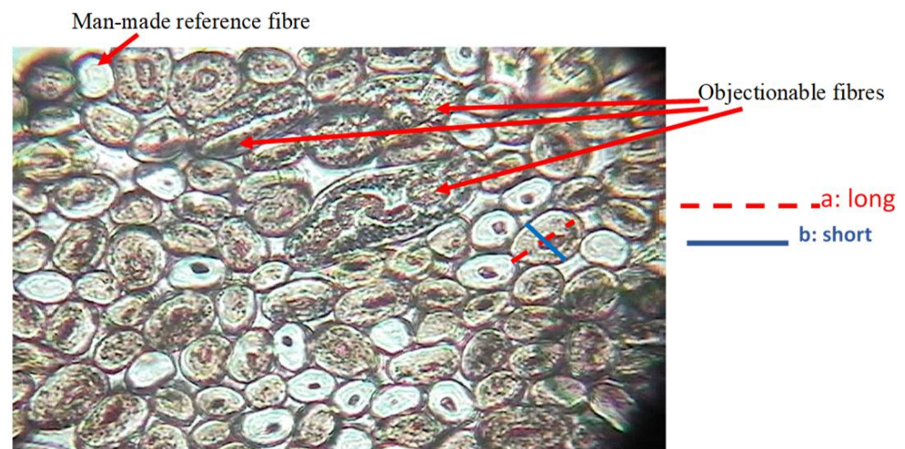
Figure 1. A microscopically pictured cross-section of the fibre sample with measurement indications as the a and b axes.
